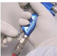
5. The spray pattern size and shape is a result of the influence of all of the air jets from the Air Cap and the quantity and speed of the fluid jet from the Fluid Nozzle. If the flow from any of these jets is uneven or distorted by dirt or damage to the holes then a bad pattern shape will be the result.
