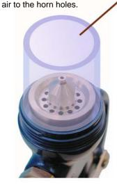
2. The amount of air going to the horn holes is controlled by the control valve on the top back of the gun.
