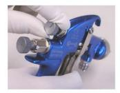
3. Air from the ring of holes in the Fluid Nozzle feeds air to the Air Cap centre annulus
